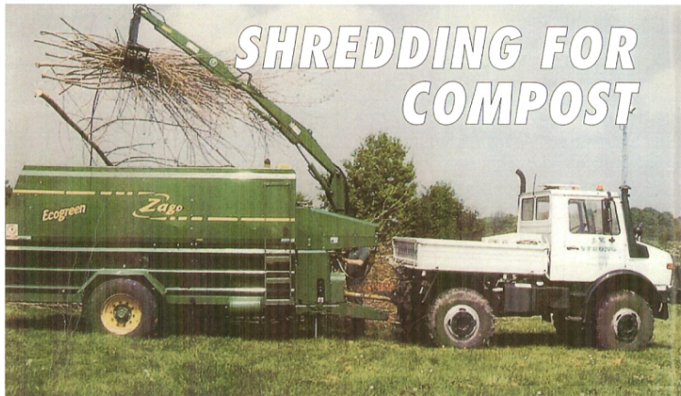
The Zago Ecogreen shredder has its own crane for loading and is towed and powered by a 160hp Unimog.
